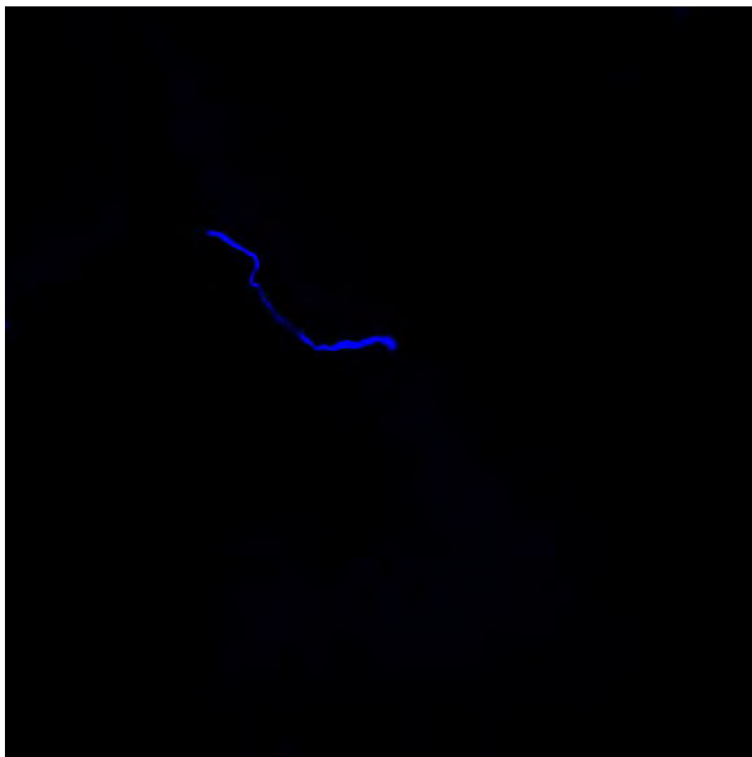
Figure 8. Microplastic (fiber) dyed with Nile Red under a fluorescence microscope (a non-plastic particle is observed partially under the fiber).
